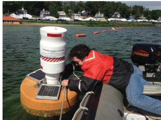
*USGS scientist Joseph Levitt secured the new buoy, equipped to monitor water quality, at Weirs Beach on Lake Winnepesaukee, New Hampshire in June 2016. Photo: Sanborn Ward, USGS*
